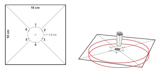
Place the paper into a Petri dish partly filled with a solvent mixture (n-butanol, acetic acid, water -4:1:1) and cover the paper with a cap.
