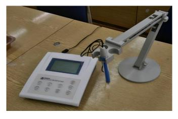
There is a pH meter with combined electrode (consisting of both the glass and the reference electrode) at your working place.
